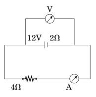
A battery of emf 12V and internal resistance 2  $\Omega$  is connected to a 4  $\Omega$  resistor as shown in the figure.
